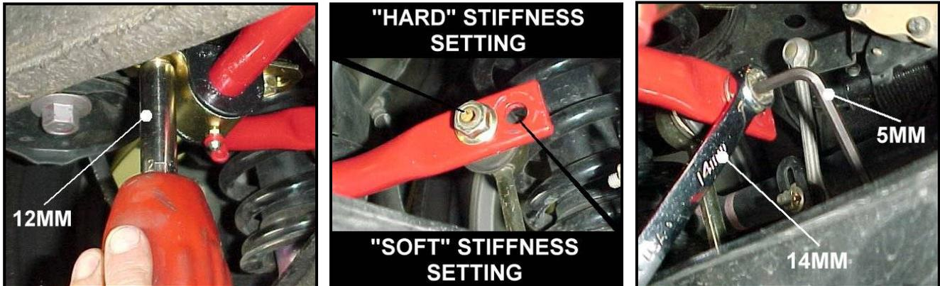
As was shown on the front bar, the stiffness of the rear bar is determined by the hole used with the end link. The hole nearest the ends is the “soft” setting and the hole towards the middle is the “hard” setting.
